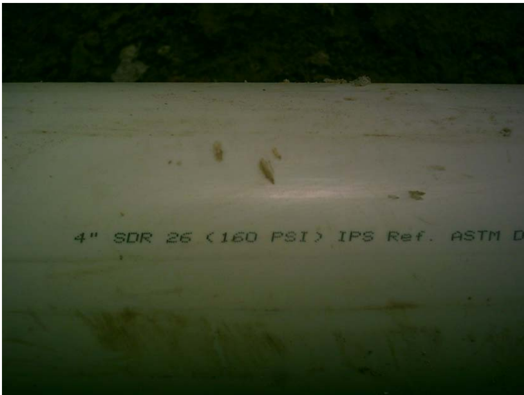
The new pipe is SDR26 PVC
